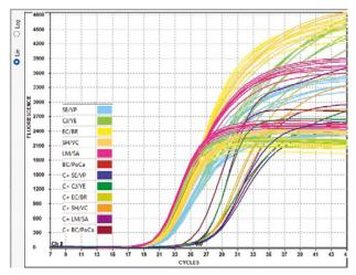
Example of real-time PCR using Lyo Blank-DNA kit for DNA detection. PCR results for food safety pathogens: 12 targets, 6 unknown samples, one PTC and one NTC control (FAM/TxR duplex assays). Time of analysis: 32 min (45 cycles).
