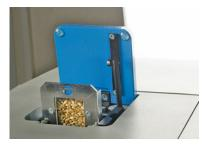
Fill the sample cell, place it into InfraLUM FT-12, choose the analyzed product in the menu and start the measurement.
